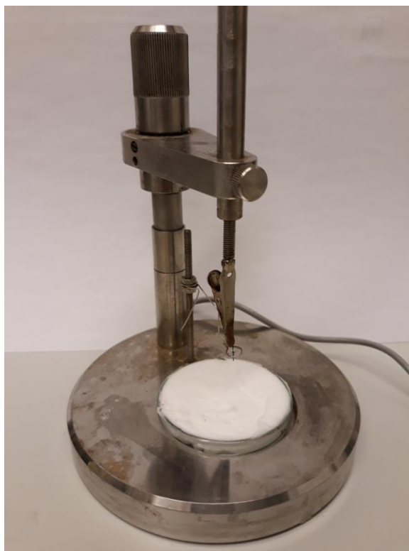
Fig. 5: Schematic of electrochemical etching of STM tips. The etched wire is held in a holder and inserted into the electrolyte membrane. The latter is held in a ring of counter electrode. When the voltage source is switched on, the wire is etched until the bottom part falls off to form a single tip. An ammeter is also wired into the circuit to monitor the current.
